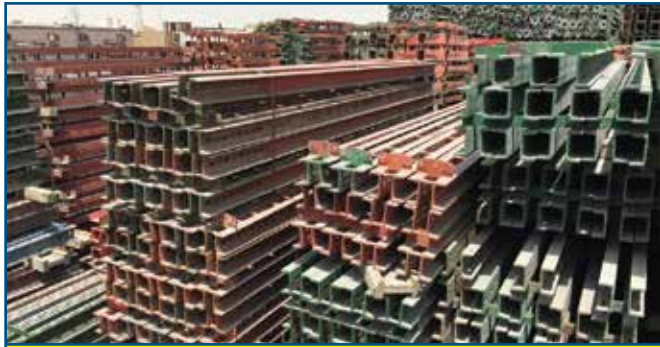
USED PERI VARIOUS SIZE SRZ WALER AND SUPPORTING ACCESSORIES (VARIO SYSTEM)
